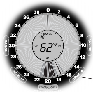
Fish at 17' and either baitfish or larger fish at edge of cone at 16'.
