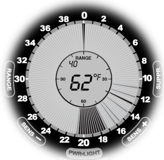
17' bottom with low dense weeds changing to sparse weeds at 14', a possible fish at 13' and clear water from 11' up.
