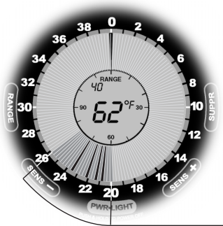
A sloping bottom causes a "Dead Zone". In this illustration, the Dead Zone starts at 20' and continues to 26'
